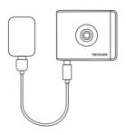
Connect TinyScope CAM with WIFI module.
