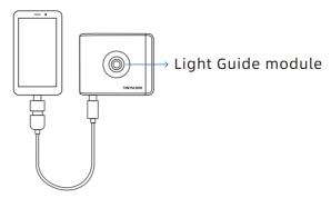
Plug the adaptor into the USB port of the data cable (then both ends of the data cable are Type-c ports). Plug two ends of the data cable that has been connected into the port of your smart phone and TinyScopeCAM respectively. After successful connection, the light guide area of this product will illuminate.
